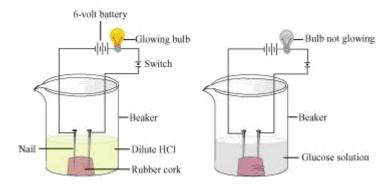
Result. HCl dissociates into H<sup>+</sup> and Cl<sup>-</sup> ions. These ions conduct electricity in the solution resulting in the glowing of the bulb. On the other hand, the glucose solution does not dissociate into ions. Therefore, it does not conduct electricity
